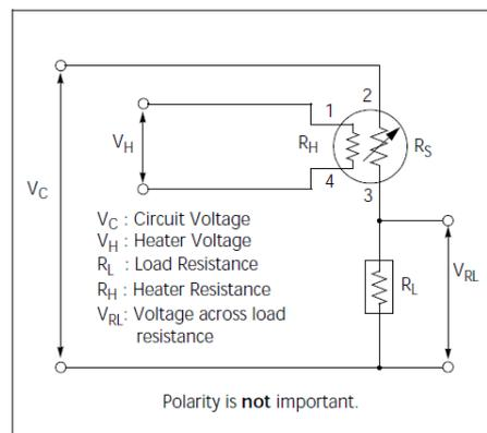
Fig 2. Standard circuit
