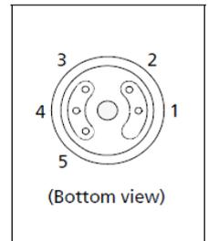
Fig 1c. Pin Layout
