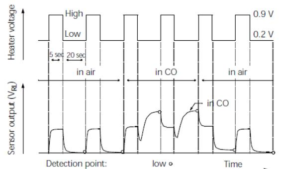
Fig 2 SB-95-12: Operating conditions and output signal
