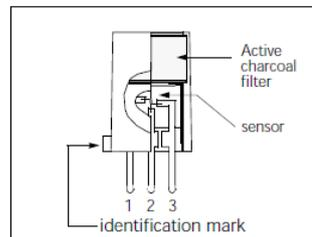
Fig 1c. Pin Layout
