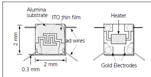
Fig. 1 Sensing Elements
