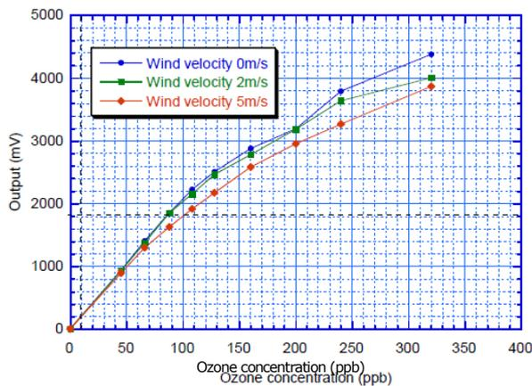
**Fig. 5 Wind influence (Output range: 0 to 5V)**
