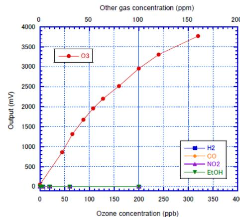
Fig. 3 Monitor sensitivity characteristics (Output range: 0 to 5V)
