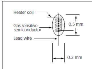
Fig 1. Sensing element
