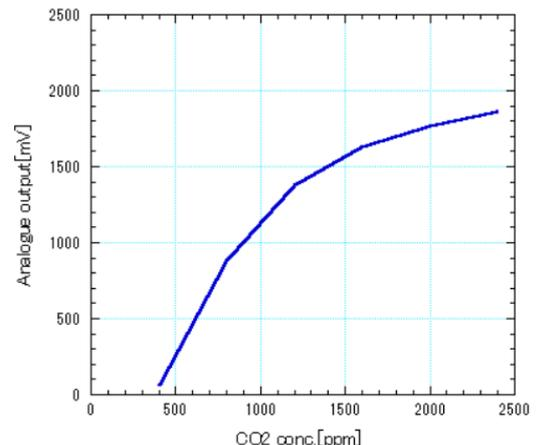
Fig 4. Converting analogue output to CO<sub>2</sub> concentration
