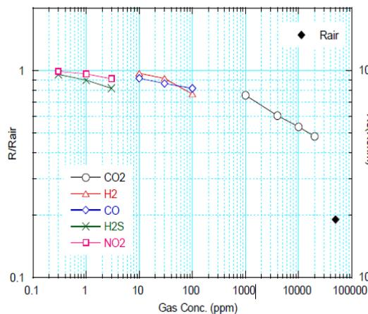
Fig 3. Cross sensitivity (SB-AQ6A)
